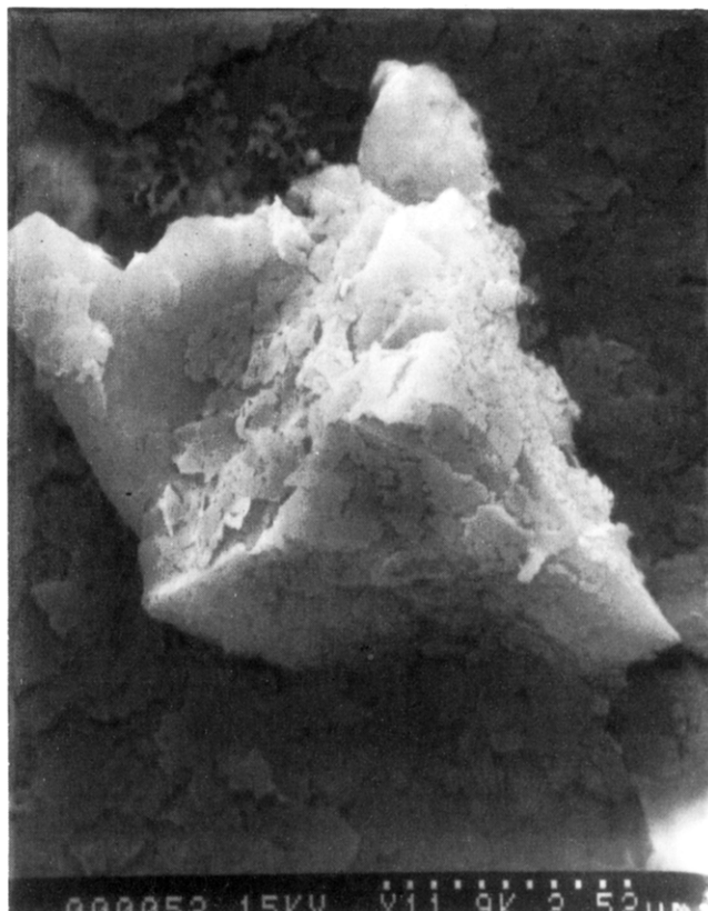
Figure 6. (1) KTP microcrystal at early stage of decomposition. (2) KTP microcrystal at later stage of decomposition.
